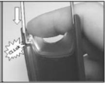
Push the Metal Slide onto the snap on the opposite side. A click should be noticed.
